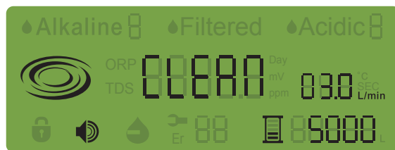
After using Acidic 3, automatic cleaning using filtered water to void drinking strong acidic water
